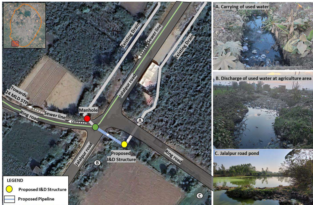
Image 6-4: Showing discharge and proposed I&D location at Jalalpur Road
