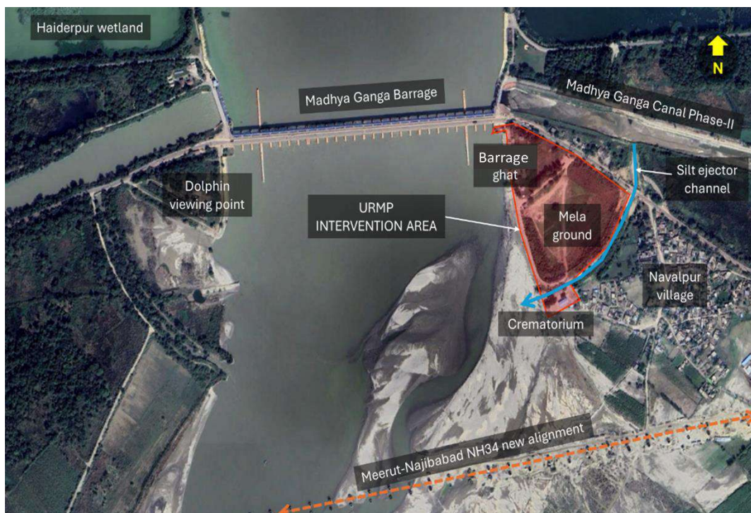
Image 6-22: Key developments around URMP intervention area at Madhya Ganga Barrage
